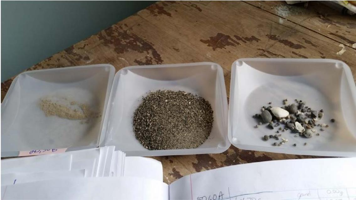
Figure 9. Sediment went through 2 different sized sieves (2mm, and 0.5 mm) and was separated by size to determine the percent gravel (right), percent sand (center), and percent silt/clay (left) for each site. This was done for three samples taken at each site.
