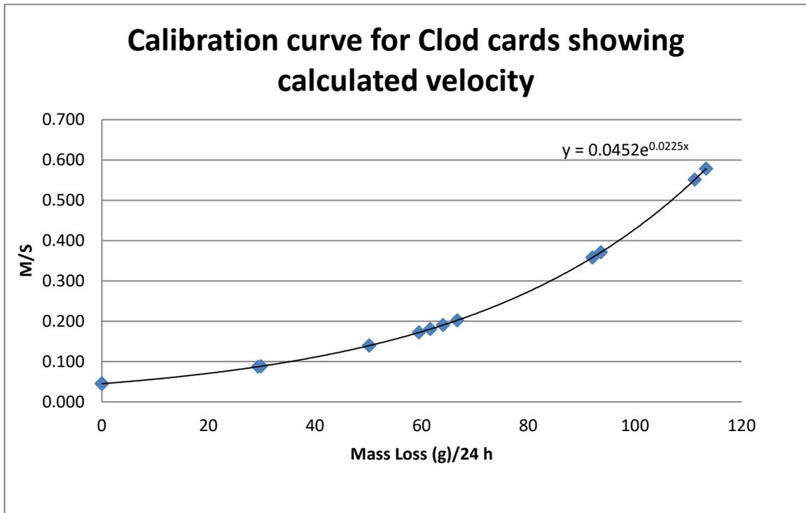
Figure 7. Calibration curve used to find the velocity of the water (m/s) from the mass lost in 24 hours (g/24 h). This calibration curve was determined by taking the amount of mass lost at a given velocity and a given time.
