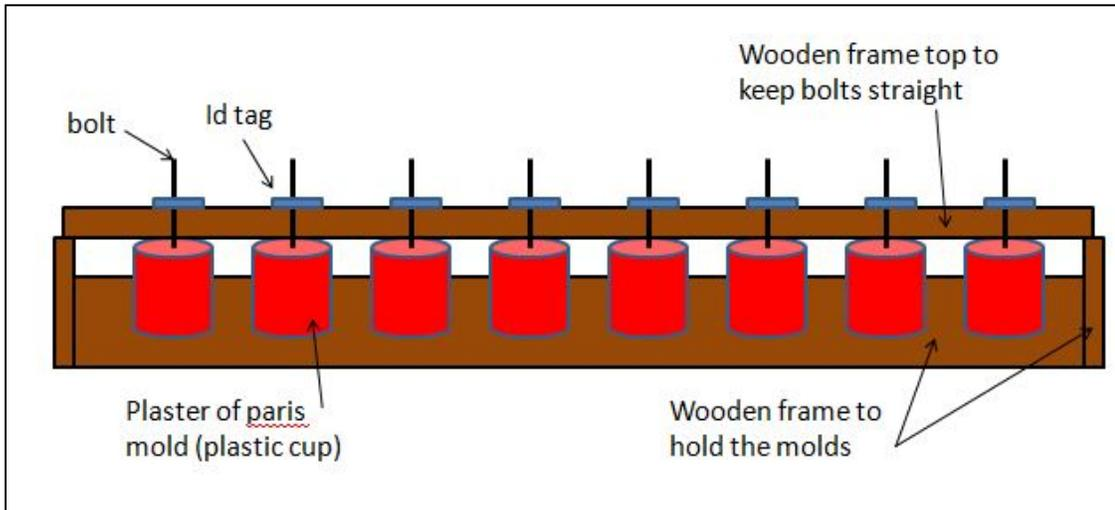
Figure 5. Wooden frame used to make the clod cards. The base had slots to hold plastic cups used as a mold for the plaster of Paris, at the top another wooden board kept the bolts and id tags straight and in the proper position as the plaster of Paris hardened.
