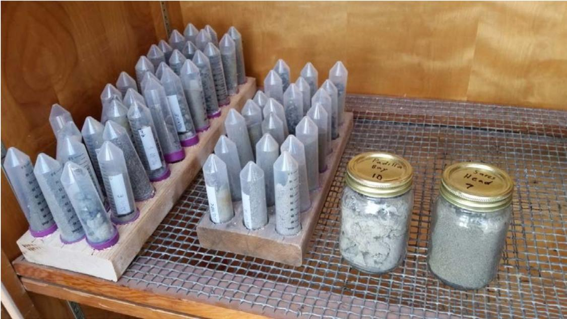
Figure 8. Sediment cores were taken with falcon tubes with a hole drilled in the small end to allow water to exit as the tubes were pushed mouth-first into the sediment. Once the sample was taken the lid was screwed back on and then they were stored and transported like this until analysis could be done
