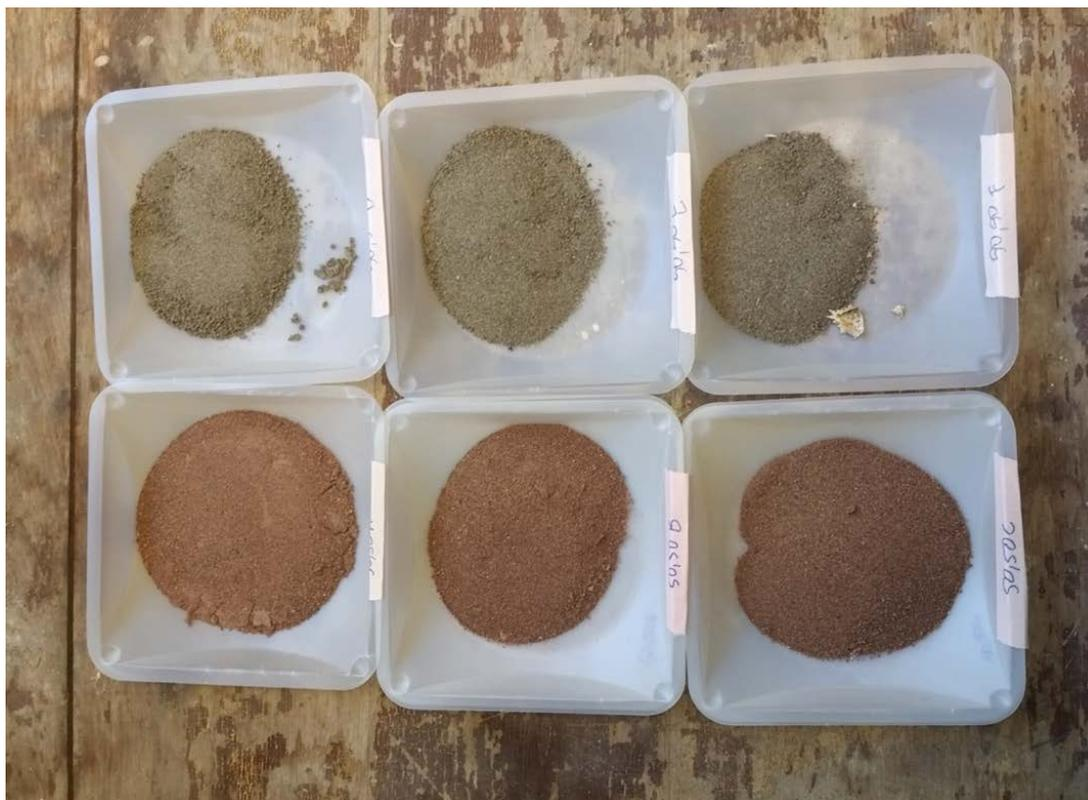
Figure 10. Sediment samples from an individual site. The top three trays contain samples that haven't gone through the muffle furnace. The bottom three trays contain samples that went through the muffle furnace. There was a color change in the sediment as the organic material was burned off.
